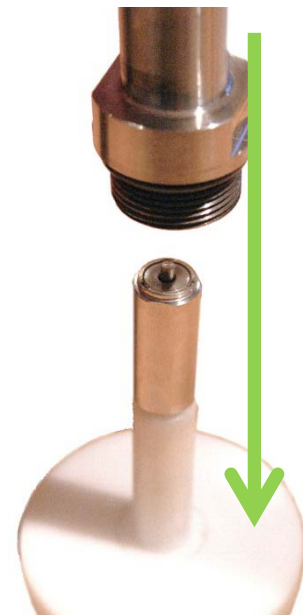
Valve armature gauge
